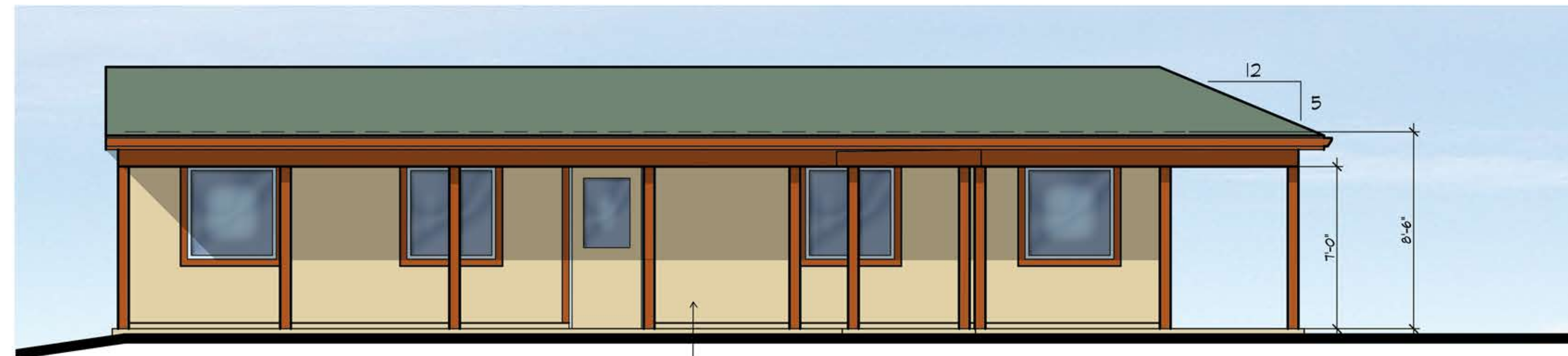
HARDI PANEL STUCCO FINISH COLOR TO MATCH PRESCHOOL BUILDING. WEST ELEVATION SCALE: 1/4" = 1'-0"
